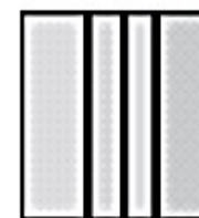
Four Layer Coextruded Structure
