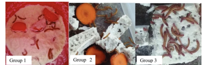
The larvae of T. molitor (mealworms) reared in the presence of corn flour (Group 1), polystyrene and carrots (Group 2) and polystyrene only (Group 3)
